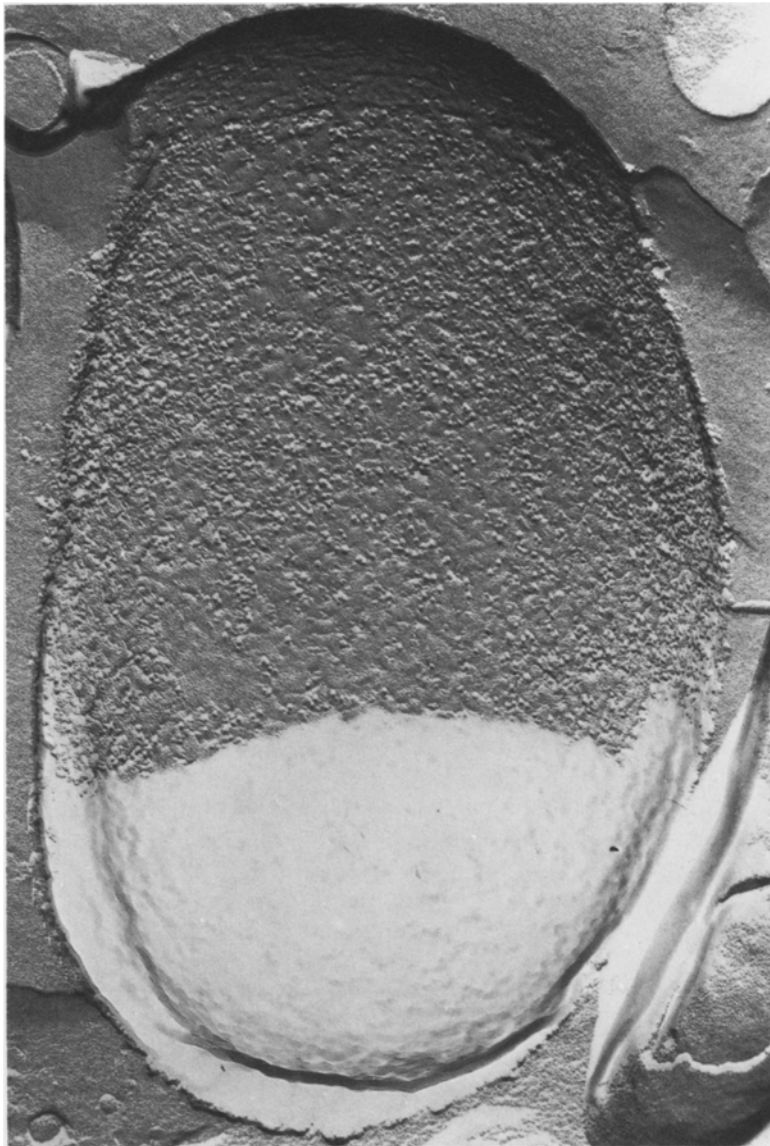
Fig. 3. Freeze-fracture replica of an MIP26 reconstituted vesicle. In some experiments large vesicles can be seen which are heavily incorporated. In these vesicles most of the particles and pits are grouped into disordered arrays similar to those of intact junctions (Fig. 2, inset ). \times 88,000
